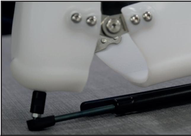
**3.4** Re-attach the **Gas Spring** to the Gas Spring Nipple. It is advised to place the CCD Lever Kit onto a hard surface (table or workbench) and press the **Gas Spring Boss** and Nipple which is attached to the CCD Shell into the **Gas Spring**.
