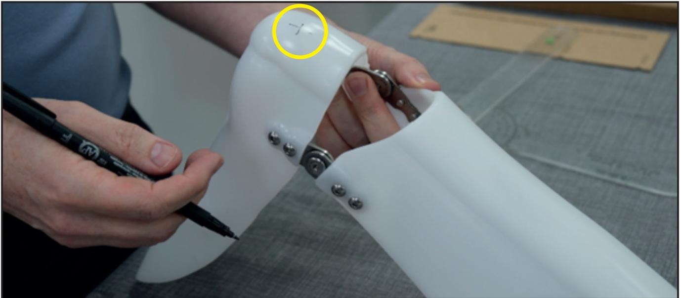
**2.3 (continued)** The marking should be in-line with the CCD shell strengthening rib. This will be the first hole position and sets the location of the **Gas Spring Boss**.
