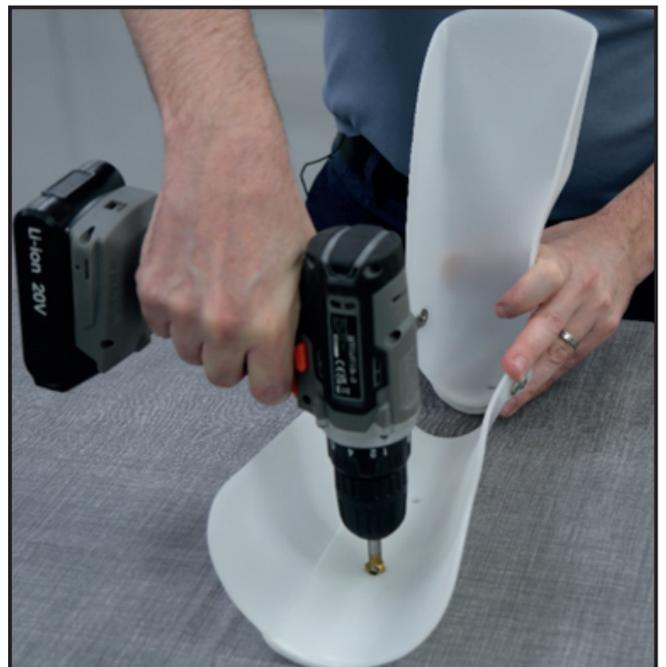
**2.12** Use the Counter Sink Bit and Hand Drill to remove any burrs from both sides of the drilled holes. Apply a 3mm Countersink to the inside face of the CCD Shell to all 3 holes.
