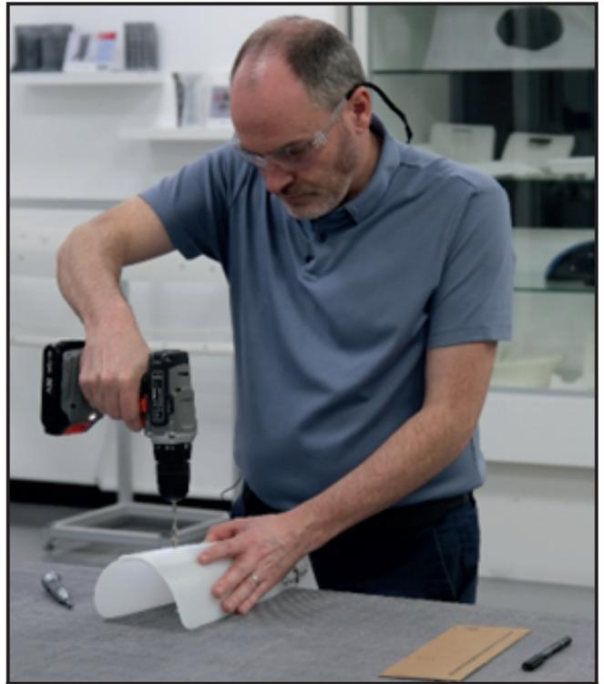
**2.11** Use the Hand Drill and 5.5mm Drill Bit to drill the x3 marked hole positions.
