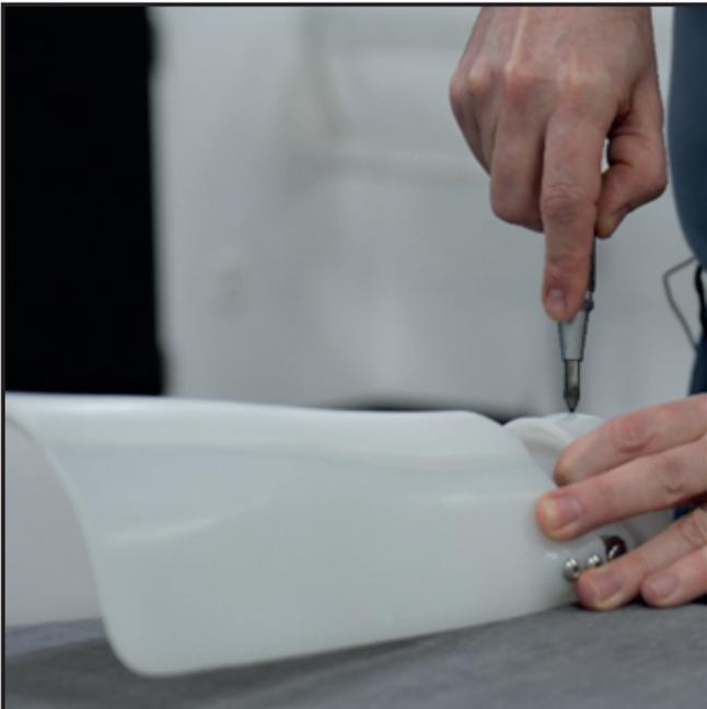
**2.10** Use the Centre Punch to indent the x3 confirmed hole positions on the CCD Shell.
