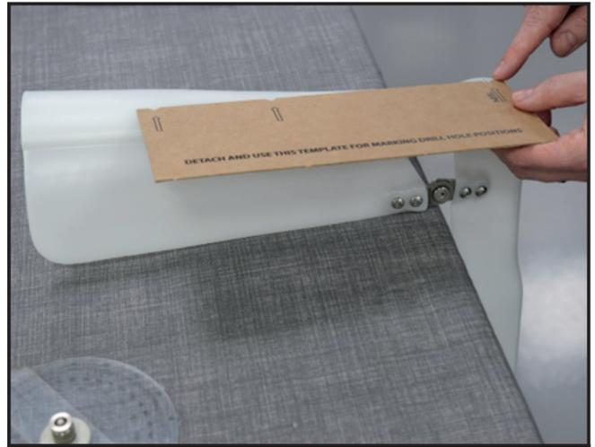
**2.7** Place the CCD on a work surface with the foot section over hanging the edge of the working area (being careful not to move the ankle joint angle set in Step 2.1). Detach the template for marking drill hole positions from the kit box and align the bottom v-cut (marked "HEEL") with the cross-hair previously drawn on the CCD heel apex.
