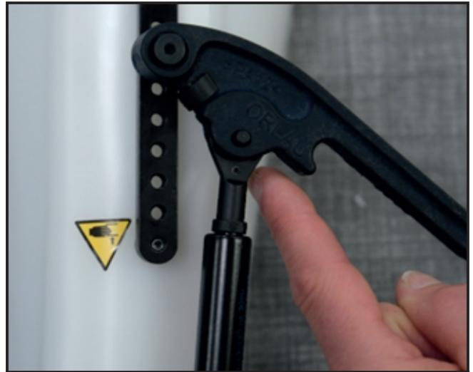
**3.5** Attach the 'Trap Point' **Warning Decal** onto the CCD Shell. Locate on the opposite side to the **Lever** near to the potential trapping point (which is where the **Rod End** contacts with the **Lever**).
