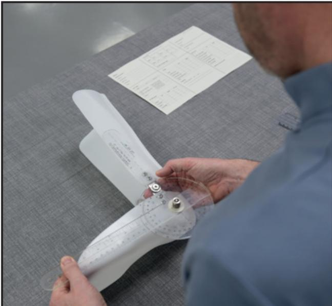
**2.6** After marking the CCD Shell check the angle set in 2.1 has been unaltered using the Goniometer.
