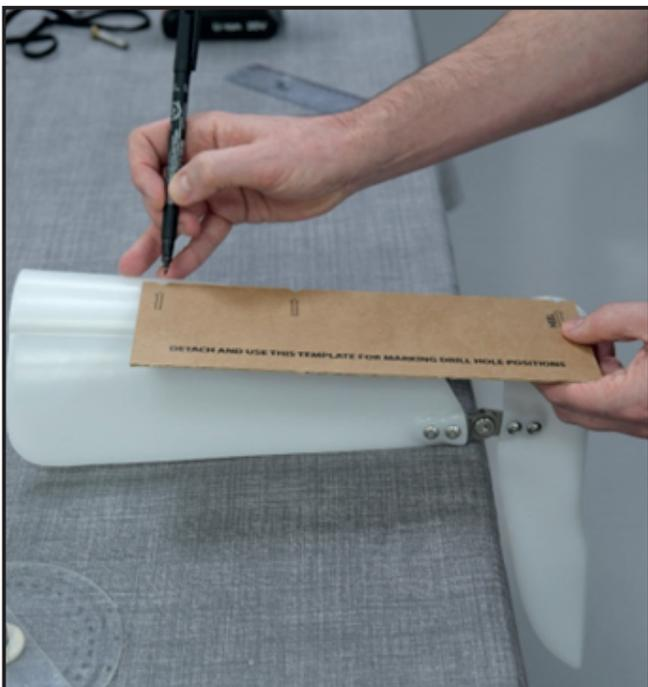
**2.8** While holding the drill position template aligned at the heel position, mark the remaining x2 positions in the v-cuts also indicated by arrows on the template.
