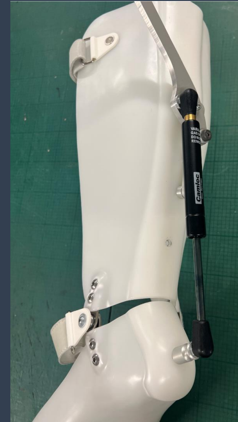
Off-centre loads deformed the pivot point
