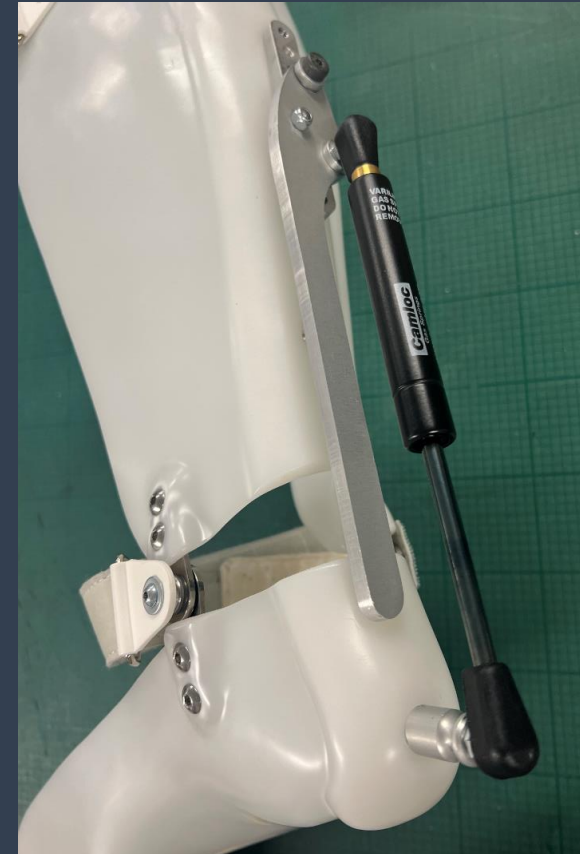
Off-centre loads deformed the pivot point
