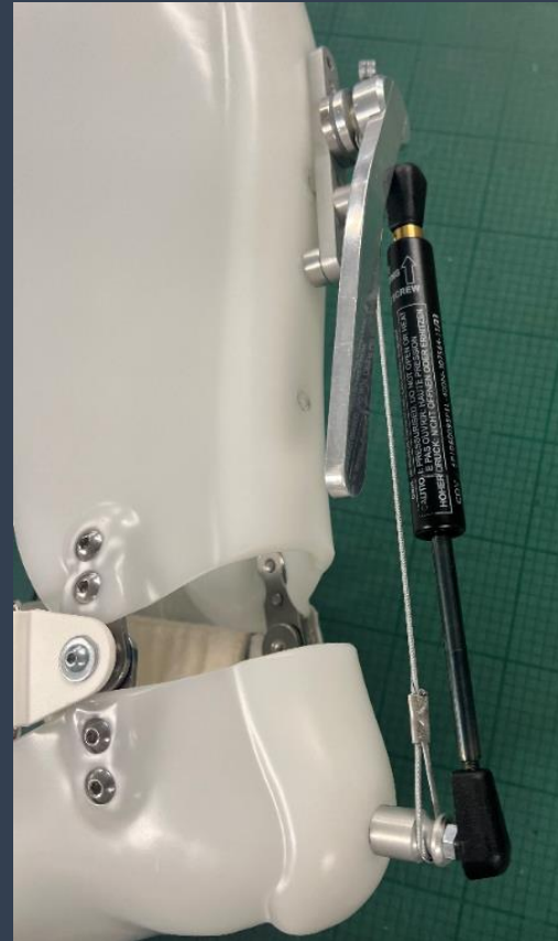
Complicated to machine and the cable kept failing
